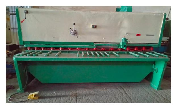
Cutting Capacity: 10mmCutting Length: 3000mm
