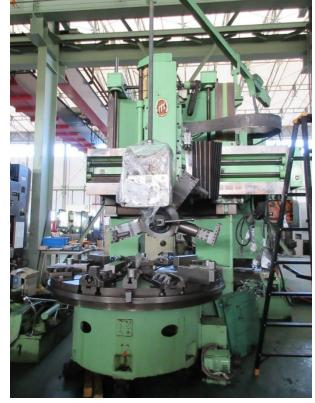
Operating Voltage:AC 100V,DC 24VTotal Power capacity:75KVAMain motor(Ac motor):37/30KwCross rail vertical movement motor:3.7Kw x4p)Turret motor (Ac servo motor) x.2:a30X,Z speed box lubricating oil pump motor:0.75Kw x 4PHydraulic pump motor(including hydraulic balance):0.75kw x 4PLubrication oil pump motor:0.75Kw x4P
